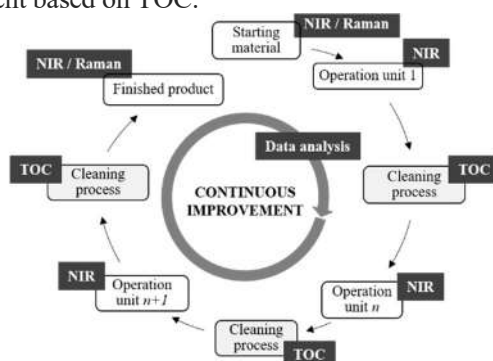
Figure 3. Continuous improvement based on PAT advanced manufacturing.
