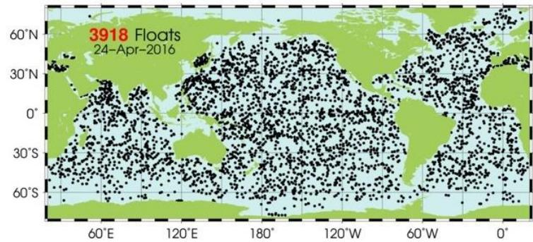
**Figure 6.2** *Left:* Preparing an Argo profiling float for deployment (photo: A Piola). *Above:* Current global deployment (from <http://www.argo.ucsd.edu>). Although coverage is generally good, there are still gaps associated with ice cover in the Arctic and Southern Ocean, and depth profiling is limited to ~2000 m.
