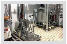
The Centre for Research in Food Technology (CERTA-UAB) has launched the first pilot and demonstration plant for packaging liquid foods using Ultra High Pressure Homogenisation (UHPH). This technology, which has emerged from the research at the university, allows the stable conservation of juices, dairy, wines and stock in tetrabriks at room temperature without the need for additives.
