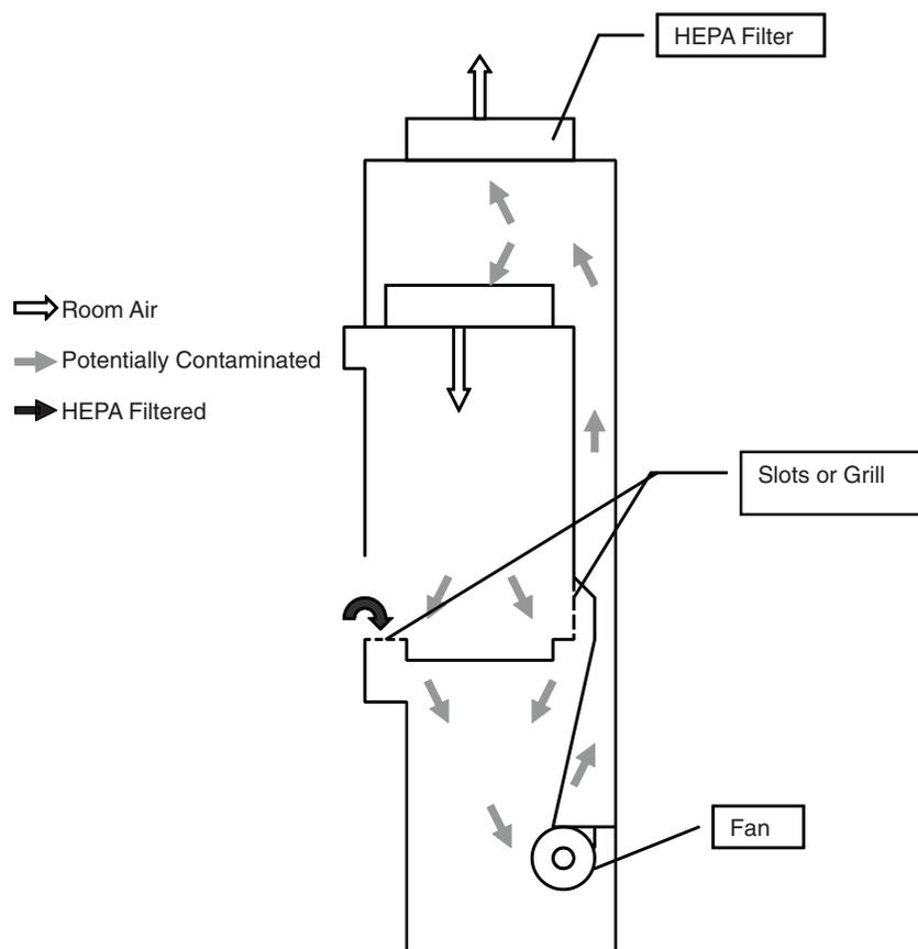
**FIGURE 9.13** Example of a Class II biosafety cabinet. Room air passes around the user through the grill at the front of the cabinet. Filtered air passes into the cabinet over the materials, providing a clean environment for the materials in the cabinet. Potentially contaminated air moves through the grill and slots, across the cabinet, and passes through HEPA filters.
