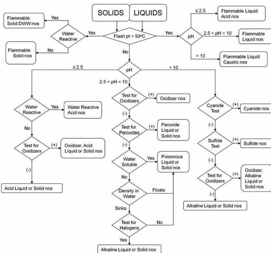
**FIGURE 8.1** Flowchart for categorizing unknown chemicals for waste disposal. This decision tree shows the sequence of tests to be performed to determine the appropriate hazard category of an unknown chemical. DWW, dangerous when wet; nos, not otherwise specified. Following categorization, select a hazard reduction procedure (section 8.D) or disposal option (section 8.B.6).
