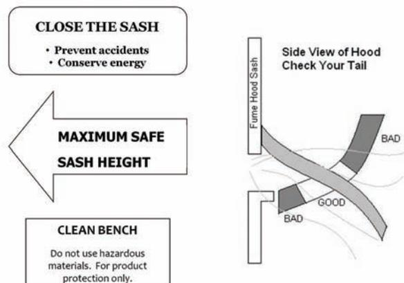
**FIGURE 9.14** Examples of postings for laboratory chemical hoods. Clockwise from top left: reminder to close the chemical hood sash, guide to checking the telltale ribbon taped to the sash of the chemical hood, reminder that a clean bench is not for hazardous chemicals, indicator showing the safe maximum sash height.
